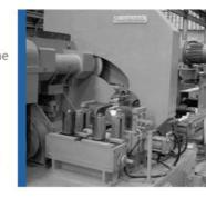
During the coating process, the pipe passes trough an online extruder to coat the pipe surface with PE/PVC film.
