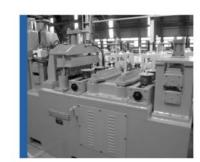
Steel Pipe Straightening Machine
